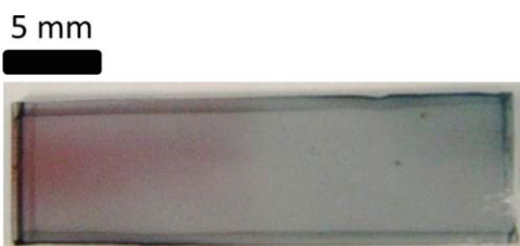
Figure 2. Glass substrate highlighting a blend of PTh (far left) and PEDOT (far right) with a large diffuse central region composed of both polymers. [Color figure can be viewed in the online issue, which is available at wileyonlinelibrary.com .]
